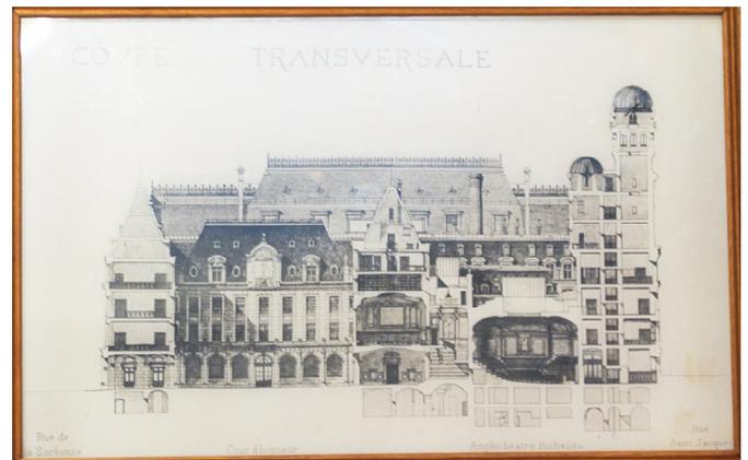
The highest part of the new buildings is the Astronomy Tower, which is crowned by two cupolas. The upper cupola was equipped with an equatorial mount supporting a 241 mm refractor for observations and a 219 mm refractor for astrophotography.
