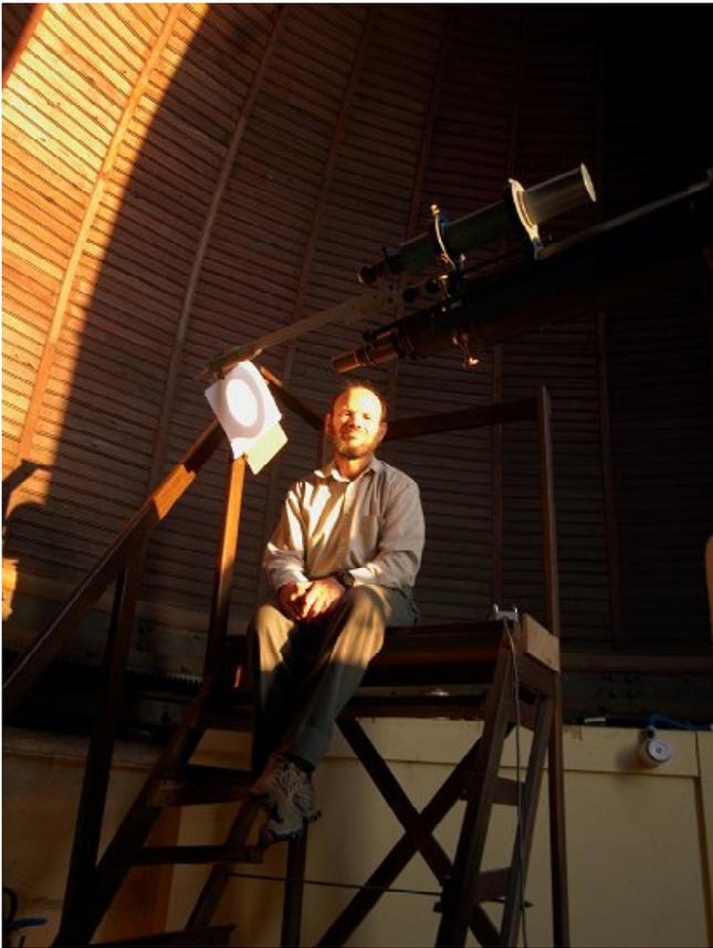
sharper than those of larger telescopes. Both the 7 ton bronze cupola and the instrument are moved by hand, except for small corrections with the right ascension motor, which also turns the instrument to compensate for the rotation of the earth.
